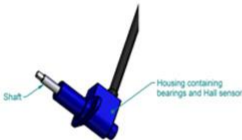
Fig. 13: Image Showing Hall Effect Based Magnetic Sensor
